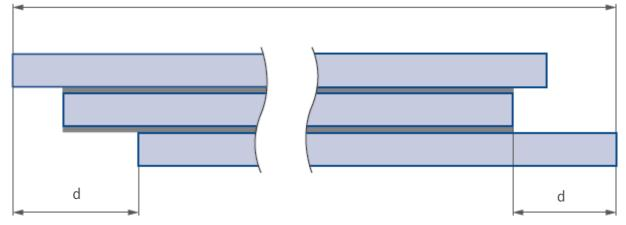
Fig. 34 Offset in cross-section of a sample laminated glass
