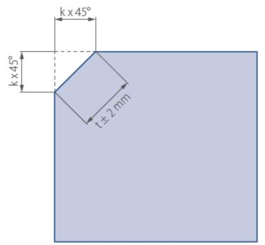
Fig. 22 Diagram of a glass pane with corner cut-off
