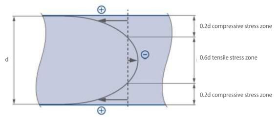
Fig. 24. Stress distribution in tempered glass (d – nominal glass thickness)
