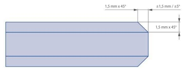
Fig. 4 Diagram of ground or polished glass edge
