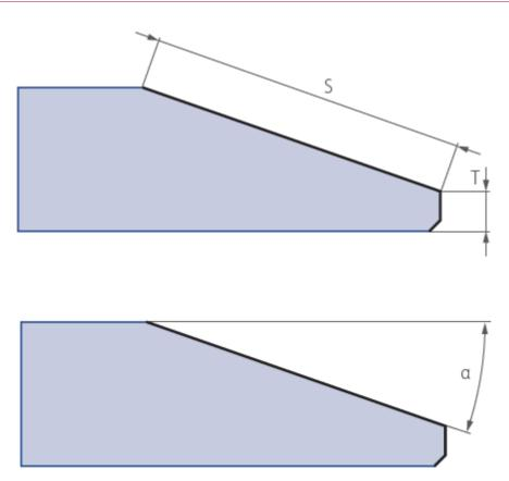
Fig. 3 Diagram of mitred glass edge
