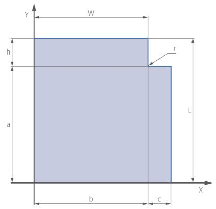
Fig. 21 Example of a corner cut-out / notch plus relevant dimensions
