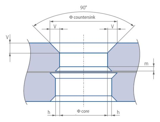
Fig. 35 Diagram of holes in laminated glass, h = 2 mm,  $m \ge 1.5 \text{ mm}$ ,  $v = (\phi_{chamf^{-}} \phi_{core})/2$
