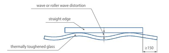
b) Measurement of wave or roller wave distortion
