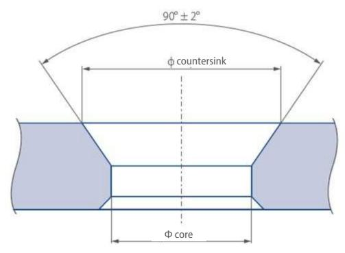
Fig. 11 Example of countersunk hole
