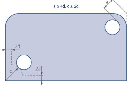
Fig. 15 Location of holes in relation to the corners
