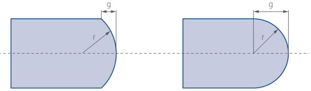
Fig. 5 Diagram of glass edge with C-edge grinding
