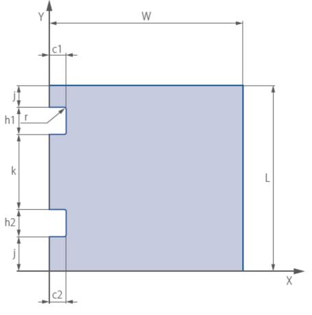
Fig. 19 Parameters of cut-outs
