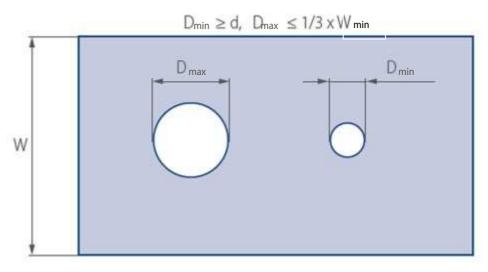
Fig. 13 Maximum and minimum hole diameters
