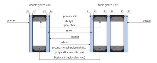
Fig. 1 Diagram of a double and triple glazed unit
