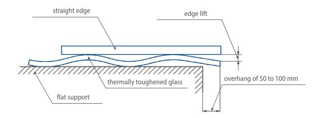
c) Measurement of edge lift
