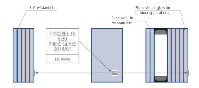
Fig. 36 Location of marking on glass for indoor and outdoor use and on glass units
