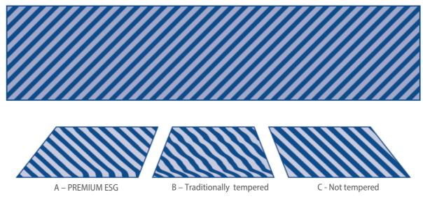
Fig. 26 Comparison of traditionally tempered and PREMIUM TOUGHENED glass
