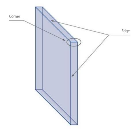
Fig. 10 Definition of edges of a glass piece
