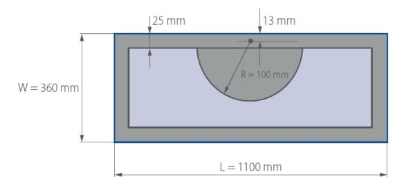
Fig. 32 An example of a specimen tested for the nature of the fracture pattern. The specified area is excluded from the assessment. The dimensions of the normative specimen shall be 360 mm x 1100 mm (W x L). Due to the manufacturing process, testing for the nature of the fracture pattern is also allowed on a sample of a different size
