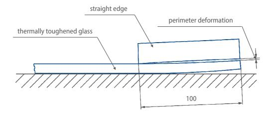
d) Measurement of perimeter deformation
