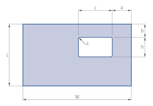
Fig. 18 Example of cut-out location and dimensional restrictions on a glass pane
