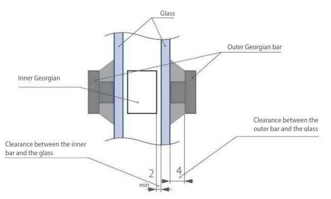
Fig. 2 Installation of inner and outer Georgian bars
