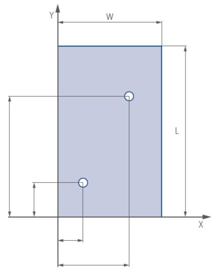
Fig. 17 Measurement of hole locations on the glass
