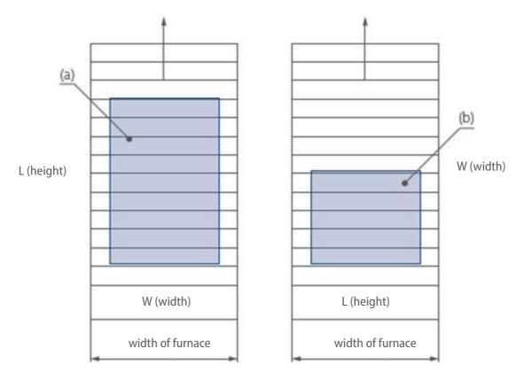
Fig. 27 Arrangement of a sample glass pane on the bed of the tempering furnace
