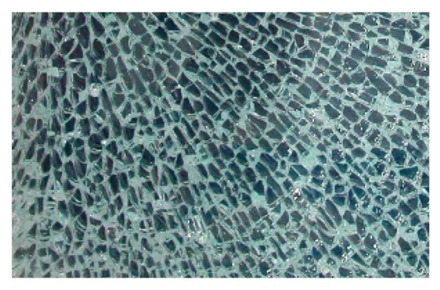
Fig. 31 Sample image of fracture (fragmentation) pattern of tempered glass with a thickness of 10mm. The structure of the cracks meets the standard requirements
